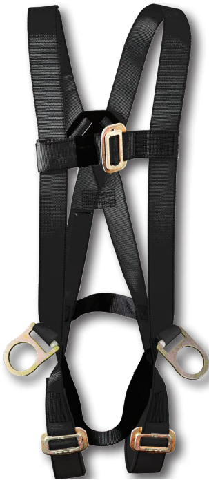
631B-HOT 3-point adjustment Kevlar® webbing Hip positioning D-rings Pass-thru leg buckles Available in sizes: S-M, M-XL
