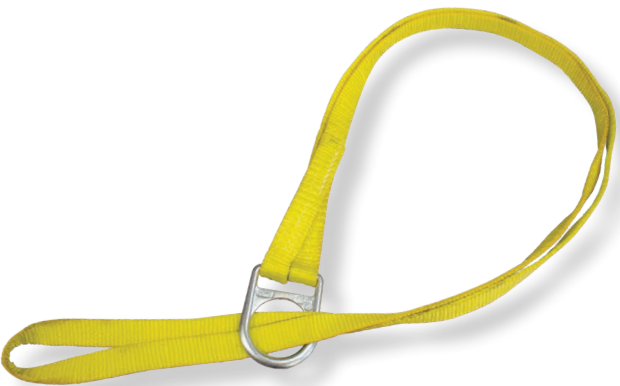
1122HD Web scaffold/pipe choker 1" 9800 lb. web, choker style, 22" long Attaches to anchors up to 3" diameter
