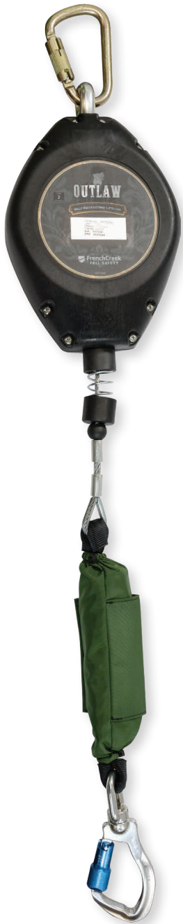
XR-50LEG 50' galvanized cable Leading Edge SRL #354-4 (1" opening) steel carabiner RL-28 (3/4" opening) locking snap Class "2" SRL
