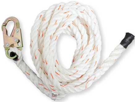
121-1S 5/8" rope lifeline #Z74 (3/4" opening) locking snaphook on one end "Whipped" opposite end
