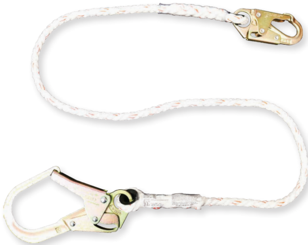
404 6' polyblend rope lanyard #Z74 locking snaphook at one end #Z136 rebar snaphook (2 1/2" opening other end)
