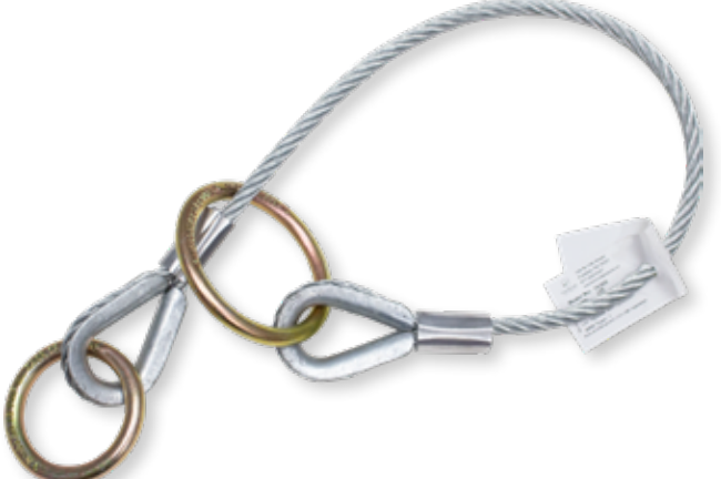
1600VC Cable tie-off adapter (pass-thru style) 5/16" vinyl coated cable 4" O-ring one end, 3" O-ring opposite end 1636VC-516 3' tie-off adapter 1672VC-516 6' tie-off adapter 1648VC-516 4' tie-off adapter 1696VC-516 8' tie-off adapter Available in additional lengths
