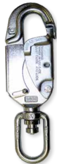
#RL-28 Steel swivel locking snaphook, 3/4" gate Impact Indicator Proof loaded to 3,600 lbs.
