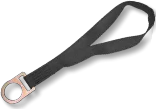
1100 HOT WORK Kevlar Web tie-off adapter Web chocker style 1 3/4" Kevlar web with D-ring 1124K 2' tie-off adapter 1136K 3' tie-off adapter 1148K 4' tie-off adapter 1172K 6' tie-off adapter Available in additional lengths
