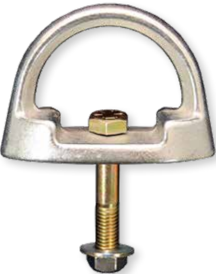
1550 D-bolt anchor (designed for anchoring into steel structure) Designed to prevent roll-out of snaphooks Grade 8, 1/2" bolt, washer, and lock nut 1 3/4" maximum steel thickness
