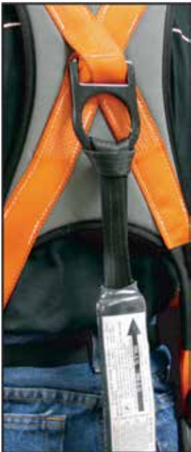
Choke-Loop 1 Pack-style shock absorber Looped End
