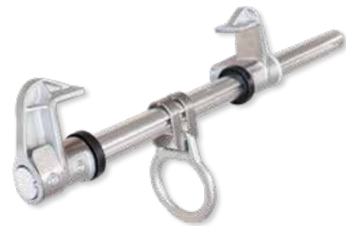
1702 Adjustable sliding beam anchor Fits flanges 3 1/2” to 14” wide, up to 1 1/4” thick Usable on top or bottom of I-beam Floating D-Ring
