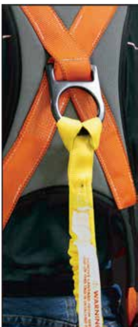
Choke-Loop 2 Internal shock absorber Looped end
