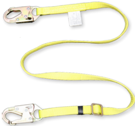
Q 450B 6' synthetic web lanyard #Z74 locking snaphooks at each end Adjustable length
